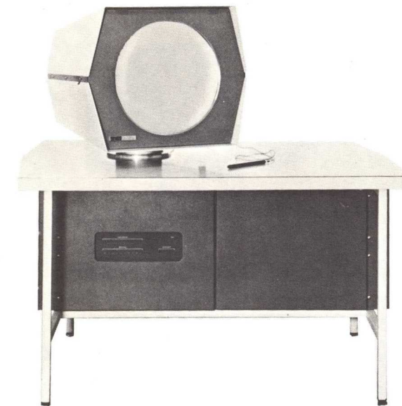
PRECISION CRT DISPLAY—TYPE 30D Displays data on a 16-inch cathode ray tube. Information is plotted point by point to form
